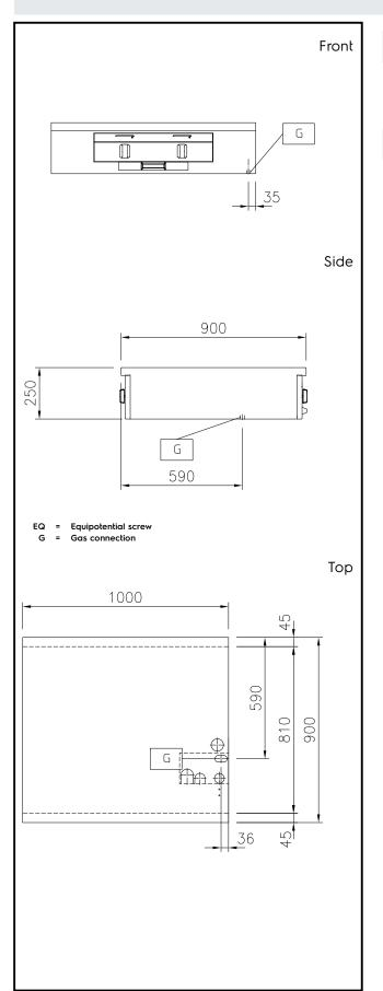
Gas Gas Power: 593317 (MCGHACJOVI) 34 kW Gas Type Option: Gas Inlet: 1/2" **Key Information:** Configuration: Two-Side Operated;Top Front Burners Power: 8.5 - 8.5 kW **Back Burners Power:** 8.5 - 8.5 kW **Back Burners Dimension -**Ø 70 Ø 70 mm Front Burners Dimension -Ø 70 Ø 70 mm External dimensions, Width: 1000 mm External dimensions, Depth: 900 mm External dimensions, Height: 250 mm
